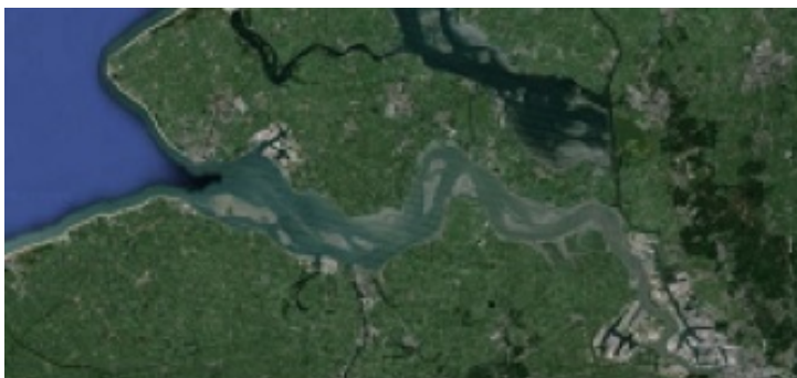
Figure 1: The Western Scheldt with many tidal flats is the main shipping route to the port of Antwerp (right lower corner). The depth of the main shipping channel is maintained by dredging. Part of this dredged material is then replaced to the
