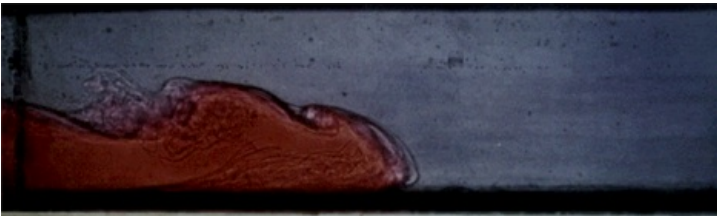
Figure 2. Propagation of the (red) salt wedge from the sea to the right across the soil. Not visible is the return flow of lighter river water to the left above the salt wedge (Friocourt et al., 2012).
