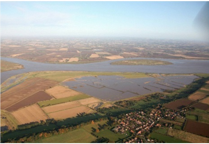
Figure 2: Aerial view of the Alkborough Flats managed realignment flood storage in operation. Photo courtesy of Environment Agency
