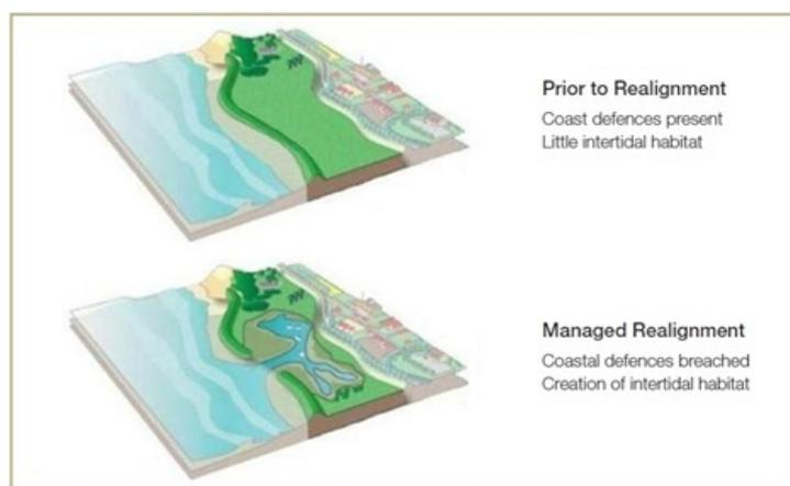
Figure 1: Managed realignment compared to the situation prior realignment. In the first picture the pre-managed realignment situation is shown with little intertidal habitat. In the second picture, the coastal defense is breached and the intertidal area increased. (Comcoast, 2006)
