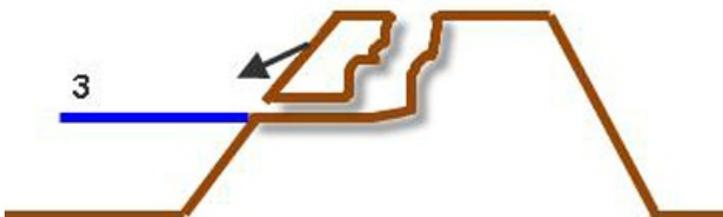
In the event of a rapid decrease in the water level, the infiltrated water drains out of the dike body. The water has created extra weight in the dike and in combination with the water pressure, could cause different failure mechanisms:
